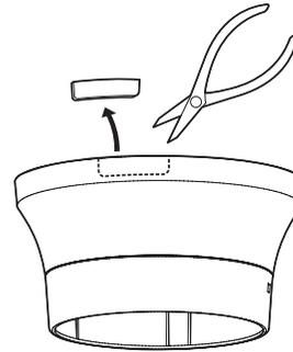
Attach the decorative cover by following step 10 of the "Wire through a hole in the ceiling" section (☞ pages 22-23). Wire through the wiring hole of the decorative cover.
