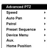
While in the PTZ mode, pressing the [PTZ] button or selecting “Ⓞ” (Advanced PTZ) in the menu displaying at the top of the screen displays the Advanced PTZ menu. Set the feature you wish to control by selecting it from the menu. Refer to the camera manufacturer’s instructions for the proper settings. Depending on the camera specifications, some features may not be supported.
