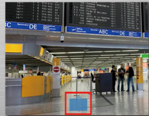
The abandoned bag is detected and indicated by red frame.
