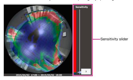
Move the "  $\mathrel{\triangleleft}$  " indicator of the sensitivity slider.
