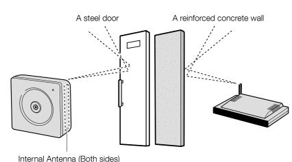
to be connected or transmission speed may become remarkably slow. In that case, it may be necessary to change the channel of a radio router or to rearrange wireless applications.
