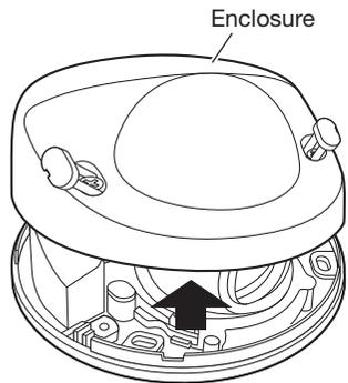
2. Detach the dome cover from the enclosure by removing the fixing screws. (Refer to the illustration described beside step 5.)
