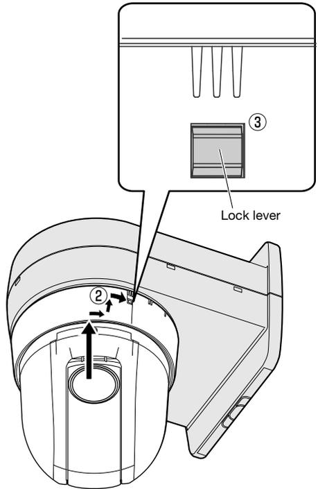
③ Ensure that the lock lever is securely inserted into the hole of the decorative cover (lower part).
