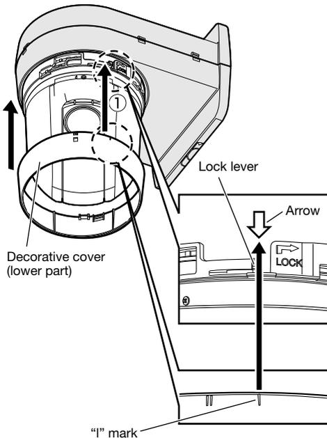
② Rotate the decorative cover (lower) clockwise when looking at it from underneath by approx. 16 degrees to insert it upward. Rotate the decorative cover clockwise by 16 degrees more to secure it.
