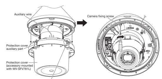
Dome fixing screw (2 pcs.) (The second screw is placed at the opposing side of this screw.)
