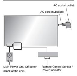
Operate pointing the remote control directly at the unit's Remote Control Sensor.
