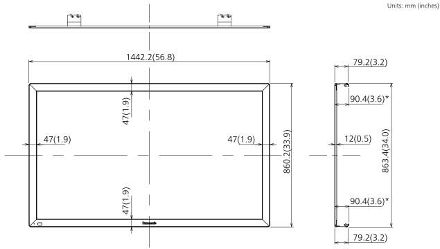
\*Dimensions may vary by the mounting set and the tightening state.
