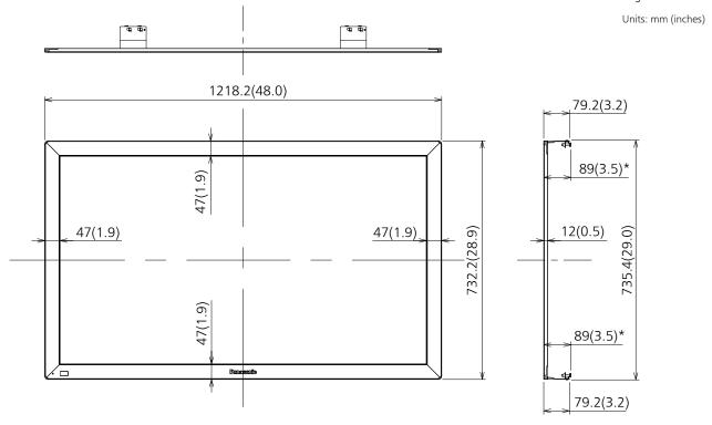
\*Dimensions may vary by the mounting set and the tightening state.
