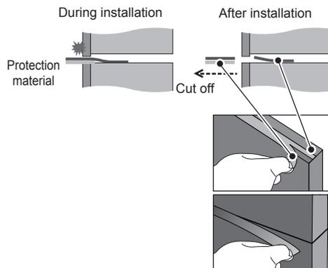
**After the displays are attached to the brackets at the back and the positions are adjusted, do not adjust the positions of the front sides using the plate, etc.**
