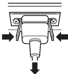
Unplug the connector pressing the two knobs.
