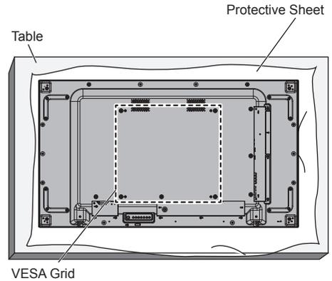
1. Lay a protective sheet on a flat table beneath the screen surface so as not to scratch the screen face.
