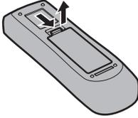
2. Insert batteries - note correct polarity (+ and -).
