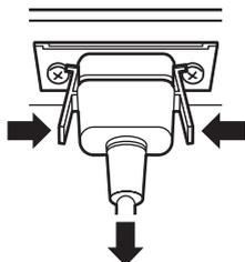
Unplug the connector pressing the two knobs.
