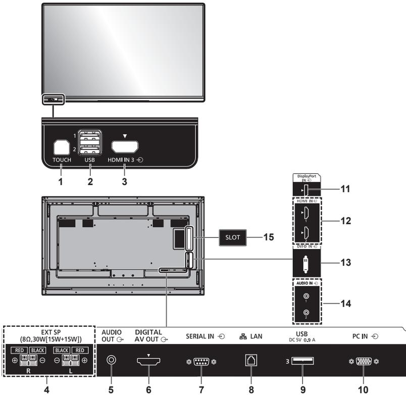
**1 TOUCH (USB):** It is connected to a PC for using the touch panel.
