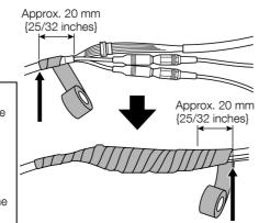
• Install the connector and cable connection parts in locations where they aren't regularly exposed to
