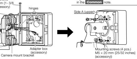
• When wiring cables on the side, use a nipper to cut open a side cable access hole of the camera mount bracket cover, and then pass the cable through.
