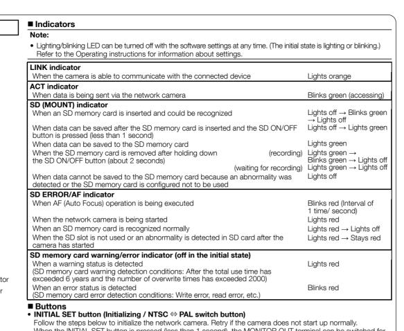
When the INITIAL SET button is pressed (less than 1 second), the MONITOR OUT terminal can be switched for the NTSC monitor ⇔ PAL monitor. The monitor out is set to NTSC in the default settings of the camera.
