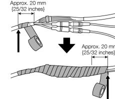
the connector parts Install the connector and cable connection parts in locations where they aren't regularly exposed
