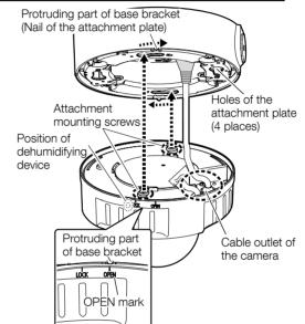
[2] Loosen 4 enclosure fixing screws using the bit (accessory), and remove the enclosure from the camera.
