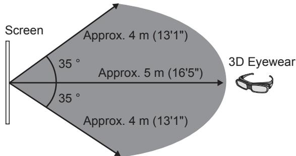
The diagram above shows the communication range under the following conditions:
