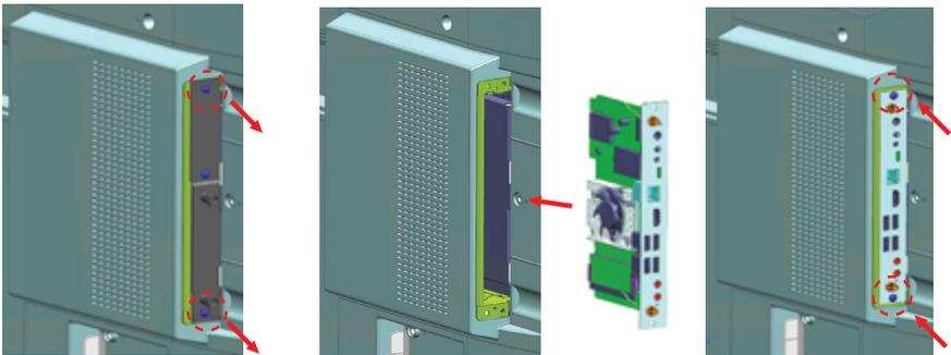
**Note:** Before attaching or removing the function board, be sure to turn off the power of the display and remove the power plug from the outlet
