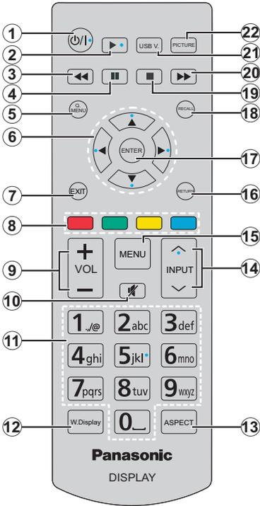
1. **Standby:** Switches On / Off the Display
