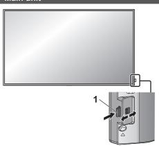
To take out/store the power indicator and remote control sensor, operate the lever on the rear panel.
