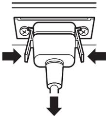
Unplug the connector pressing the two knobs.
