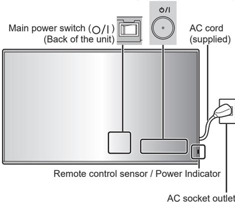
Operate pointing the remote control directly at the unit's Remote Control Sensor.
