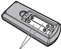
Insert batteries and close the battery cover.
