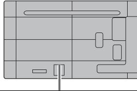
Insert the AC cord securely all the way seated on the back side of the unit.
