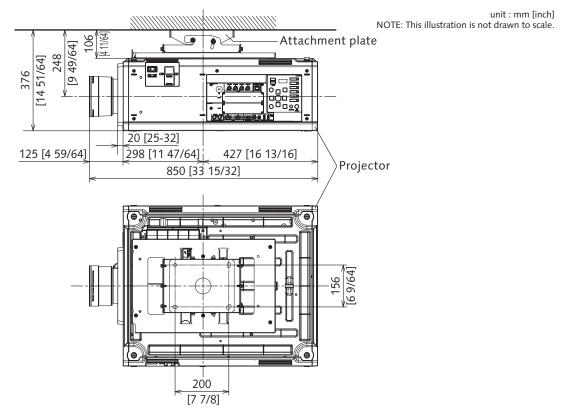
The illustration shows the ET-PKD520H ceiling mount bracket mounted on Group C projectors (PT-RQ13K/PT-RZ12K/PT-RS11K)
