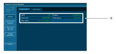
\*Displays the configuration details of wired LAN.
