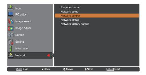
Press <ENTER> button or the ▶ button to access the submenu.
