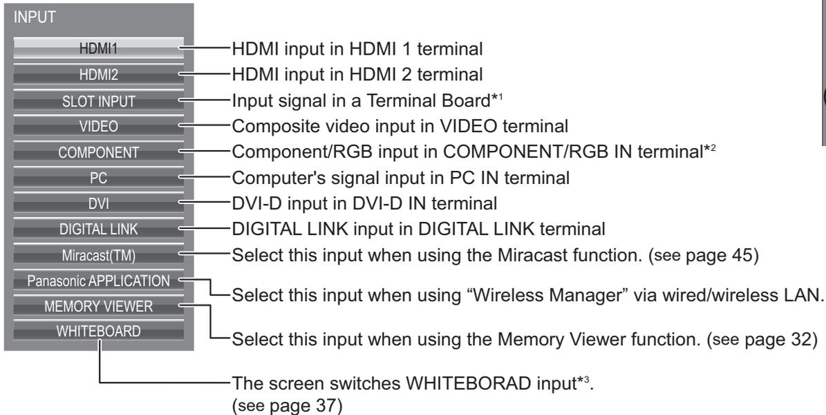
\*1 "SLOT INPUT" appears when an optional Terminal Board is connected.
