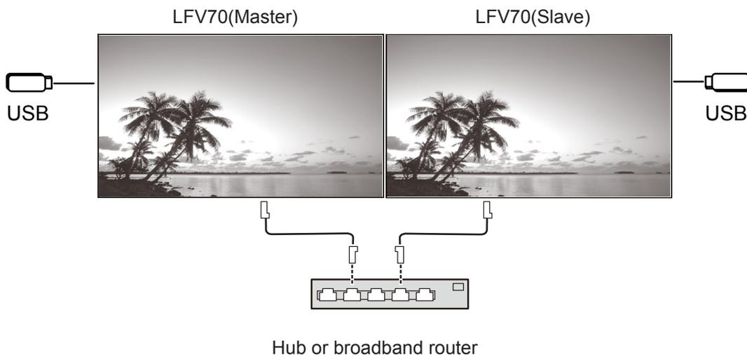
This operates with daisy chain connection of DIGITAL LINK (P20) as well.
