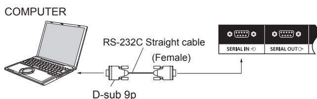
In addition, a particular LCD Display can be controlled with a PC while several LCD Displays are daisy chained.
