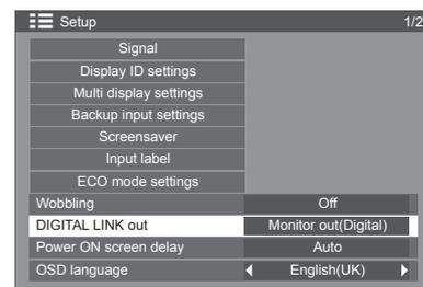
Set a signal output from the DIGITAL LINK OUT terminal.
