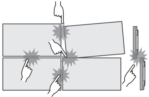
After the displays are attached to the brackets at the back and the positions are adjusted, do not adjust the positions of the front sides using the plate, etc.
