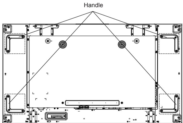
When you install a display by multi, please prepare for 0.5 mm between each display in the state of the power supply OFF.
