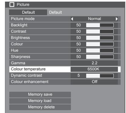
By selection the modes; from 3200K to 10700K, adjustment based on their data is available. Adjusted data is saved to "USER1" or "USER2". (It is available to select.) For the case "USER1" or "USER2" is selected, go to step 5.
