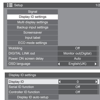
Use the ID number of each display to set up the function that individually controls several display units.
