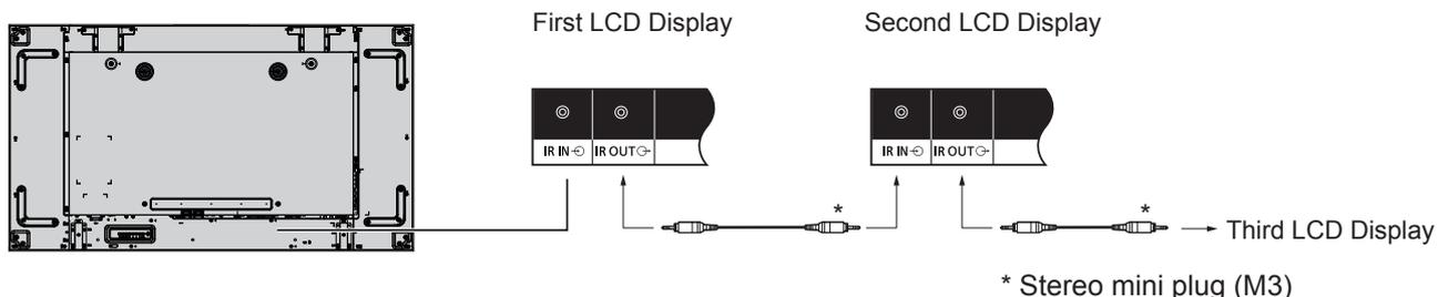
At this time, IR receiver of the Second LCD Display will not work. It is possible to daisy-chained by repeating the above connection.
