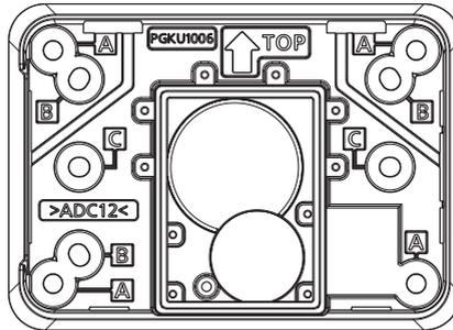
Mounting screw hole A: For standard mounting position on the wall
