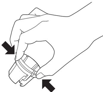
When attaching or removing the lens adjuster, squeeze the wider end of the lens adjuster as shown in the illustration to open the narrower end of the lens adjuster.
