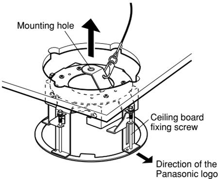
**Note:** The Panasonic logo will be directed to the ceiling board fixing screw which is secured on the side described in the illustration. When inserting the mount bracket into the ceiling, fit the bracket in the 4 mounting holes of 12 mm {1/2 inches} in diameter on the ceiling.
