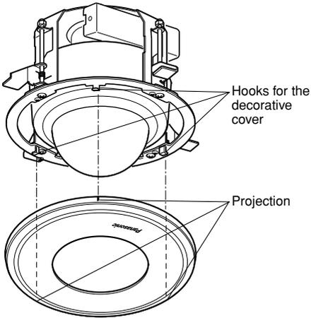
**Note:** Mount the decorative cover on the mount bracket so that the Panasonic logo is directed to the side which was determined when making the mounting holes.
