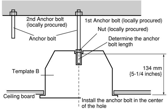
**Note:** If there is already an anchor bolt installed, the anchor bolt can be used as a 2nd anchor bolt. Make sure that the distance between the 1st and 2nd anchor bolts is 1 000 mm (3.28 feet) or less before use.
