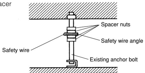
**4. Connect this mount bracket to the tip of the safety wire.**
