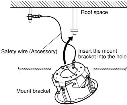
**5. Insert the 1st anchor bolt into the mounting hole of the mount bracket.**
