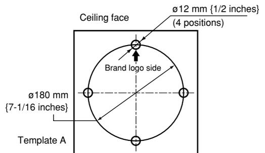
**Important:** Make a hole precisely. When the opened hole is bigger or deformed too much, the ceiling mount bracket cannot be stuck on the ceiling board securely.
