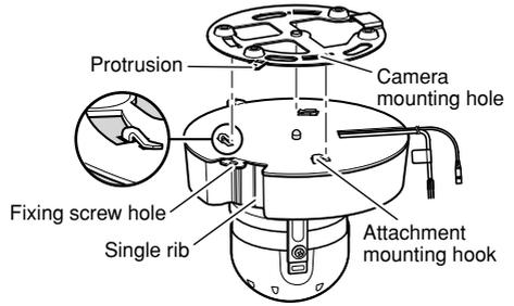
**Note:** When the camera is secured, the camera attachment protrusion is aligned with the camera fixing screw hole and the double rib on the camera.
