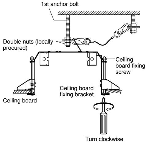
**Important:** When the ceiling board is the plasterboard, make sure that no crack was made on the ceiling board by clamping.
