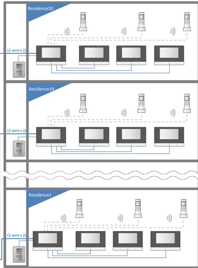
Wiring Schematic Diagram
