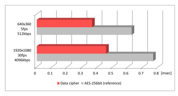
Figure 4: Encryption processing time (calculated for WV-SPN631)
