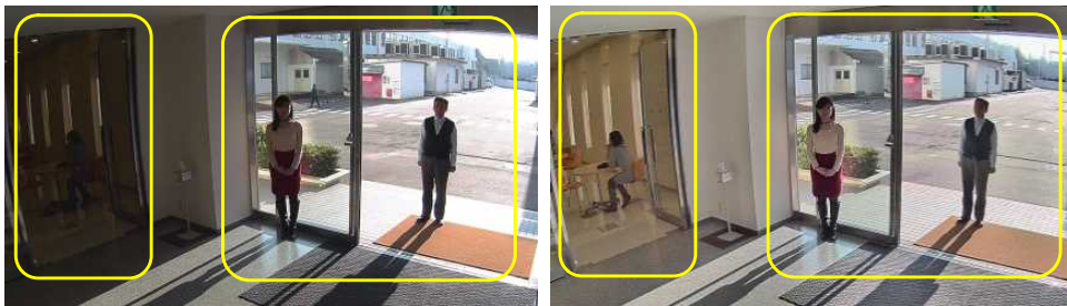
Figure 4: Entrance in backlight situation. At left, two persons are buried in black. At right, Enhanced Super Dynamic is on. Two persons at the entrance and one person at the left table can be seen clearly.
