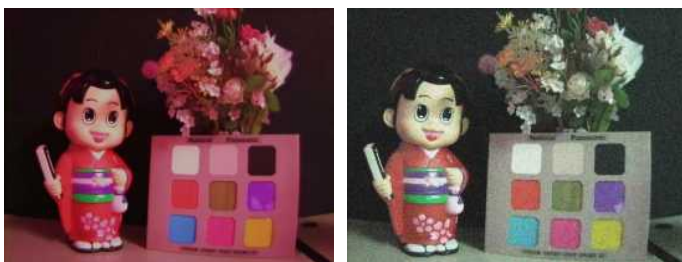
Figure 8: At left, built-in IR cut filter is removed and image is discolored in poor lighting condition. At right, the original color is recovered by Super Chroma Compensation (SSC).
