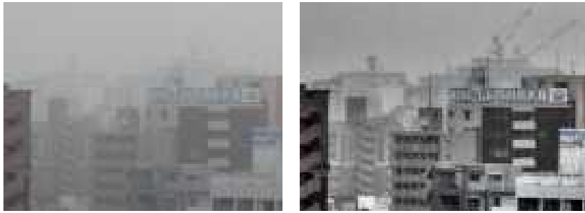
Figure 21: Buildings on a foggy day. At left, thick fog reduces visibility. At right, the image is processed through Panasonic Visibility Enhancement Software. The visibility is improved and the distant objects like cranes become visible.
