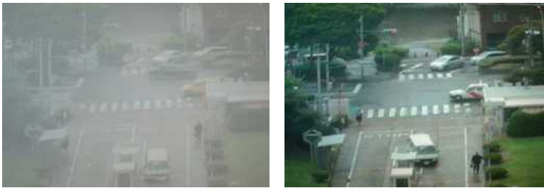
Figure 10: Outdoor gate on a foggy day. The picture on the left is taken on a foggy day with the Fog compensation off. The picture on the right is the same scene taken with the Fog compensation on and visibility is improved.
