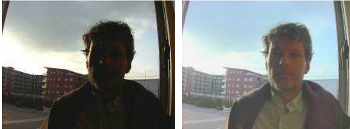
Figure 6: Person in front of a bright window. At left, the face cannot be identified. At right, Face Super Dynamic is on and his face is identifiable.
