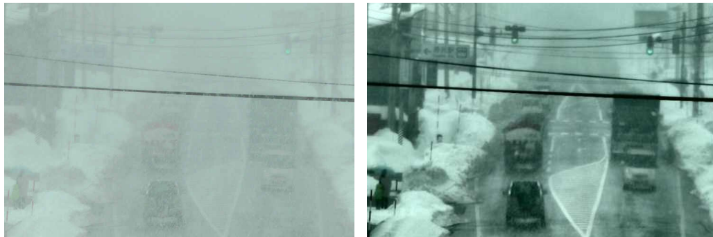
Figure 20: Road on a snowy day. At left, there is almost zero visibility due to heavy snow. At right, the visibility is greatly improved by Panasonic Visibility Enhancement Software.
