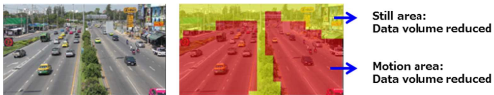
Figure 5 : Left: Original image. Right: The image is an example of separate a still area and an area with motion.
