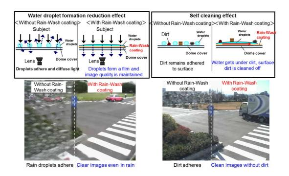
This coating technology is also applied to IR LED models. As shown below, the impact of reflection from IR projection is reduced even in IR projection environments in rainfall, enabling stable surveillance.
