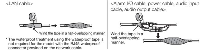
\* The waterproof treatment using the waterproof tape is not required for the model with the RJ45 waterproof connector provided on the network cable.
