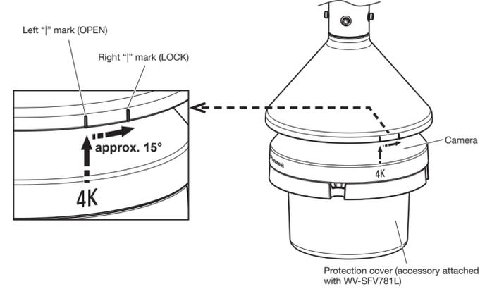
\* The direction of the camera when it is installed on the attachment plate vary by camera. For further information on the installation of a camera, refer to the Installation Guide of the camera to be installed. (The illustration below shows the example for WV-X8570N and WV-S8530N)
