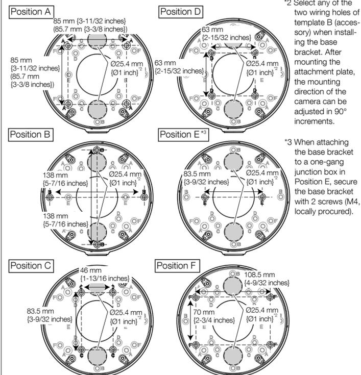
\*2 Select any of the two wiring holes of template B (accessory) when installing the base bracket. After mounting the attachment plate, the mounting direction of the camera can be adjusted in 90° increments.
