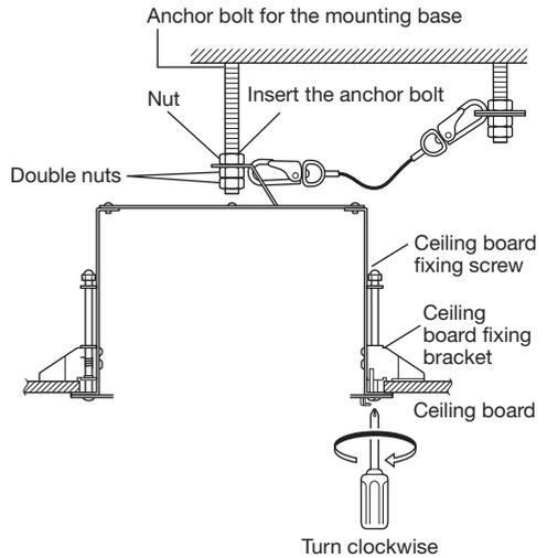
**Important:** When securing this bracket on the ceiling, make sure that the four ceiling board fixing brackets are open as shown in the figure.
