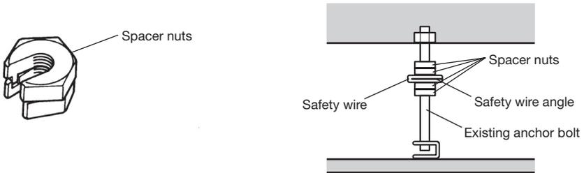
**6. Connect the mounting base to another tip of the safety wire.**
