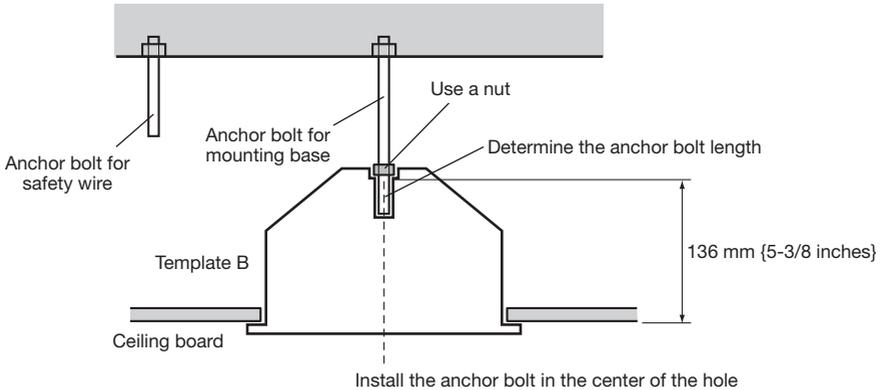
**Note:** If there is already an anchor bolt installed, it can be used as an anchor bolt for the safety wire. Make sure that the distance between the anchor bolt for the mounting base and the anchor bolt for the safety wire is 1 m {3.28 feet} or less before use.
