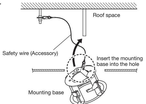
**7. Insert the mounting base into the hole made in Step 3.**
