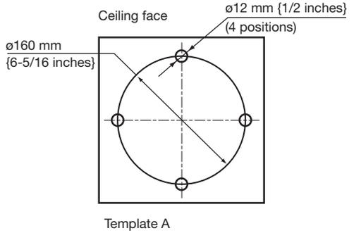
**4. Install two anchor bolts (M10 recommended) into the concrete ceiling.**
