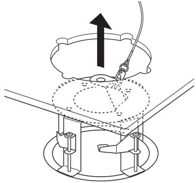
**8. Secure the mounting base to the ceiling board with the ceiling board fixing screws (4 positions).**
