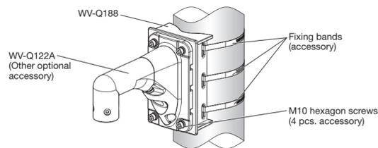
(In this illustration, fixing WV-Q122A to a pole by using WV-Q188 is taken as an example.)
