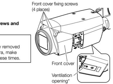
\* Do not block the surface as internal humidity is discharged through this ventilation opening. Water does not come inside.
