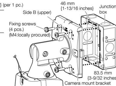
**[Type 3] Mount the camera onto the ceiling or wall using the Adapter box (accessory)**
