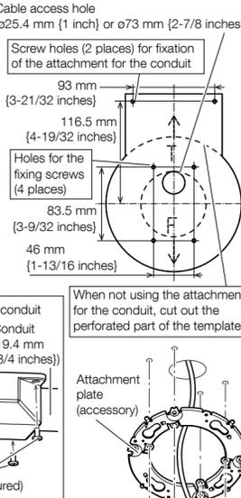
[2] Install the attachment plate on the installation surface.
