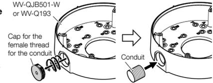
[2] Install the WV-QJB501-W or WV-Q193 on the installation surface.
