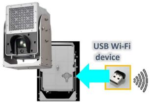
Insert USB Wi-Fi device to the USB terminal on camera
