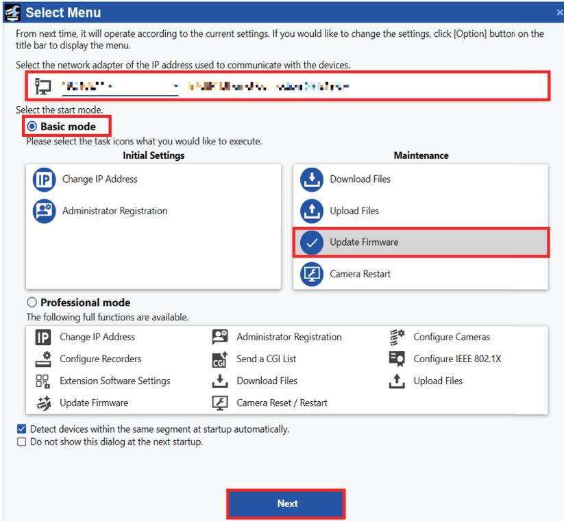
Select the IP address of the network adapter used to communicate with the WV-CU980.
