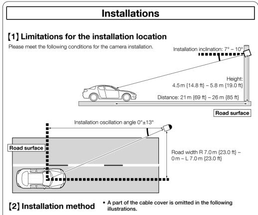
There are 3 methods to install the camera as follows. Select an installation method in accordance with the conditions of the installation location.
