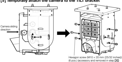
• As a temporary adjustment, roughly match the PAN and TILT and face the camera in the direction that you want to view images.
