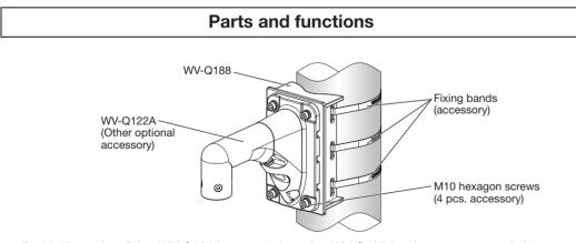
(In this illustration, fixing WV-Q122A to a pole by using WV-Q188 is taken as an example.)
