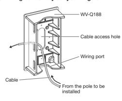
Access hole of fixing
