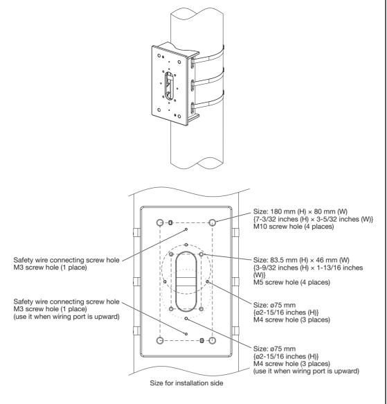
■ Size illustration for installing part of WV-Q182/WV-Q188
