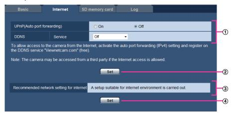
When completing the setting items in field 1, click the [Set] button 2 below field 1. The edited settings in field 1 will not be applied unless the [Set] button 2 below field 1 is clicked. In the same manner as above, click the [Set] button 4 below field 3 when completing the setting items in field 3.
