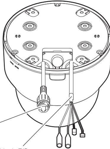
Cable de Ethernet RJ45 (WV-QCA500A)
