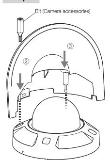
③ Temporarily secure the unit to the enclosure and rotate the long enclosure fixing screw attached to this product clockwise to penetrate the enclosure of the camera.
